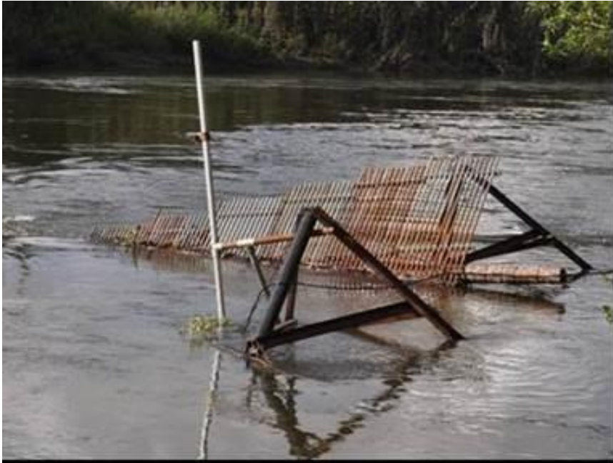
Figure 4. NB sonar unit mounted on tripod stand with diversion weir downstream of the sonar.
