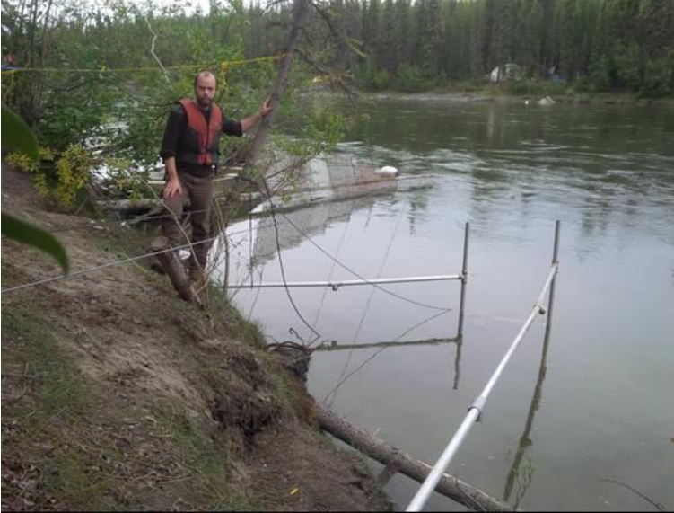
Figure 6. SB sonar unit mounted on stand with diversion fence downstream (2014 photo).
