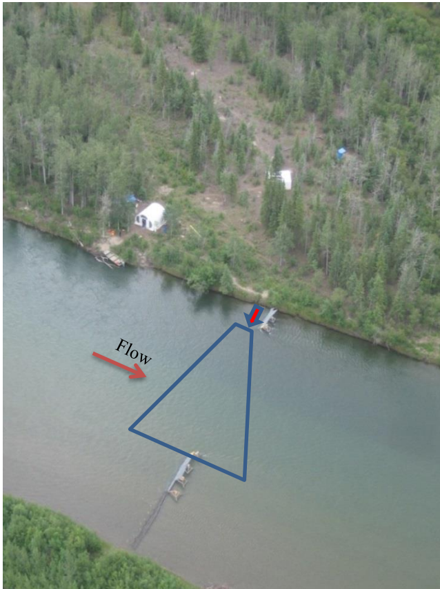
Figure 3. Aerial view of sonar station camp and partial weirs, (photo from 2010 project). Blue outline denotes ensounded portion of the river.
