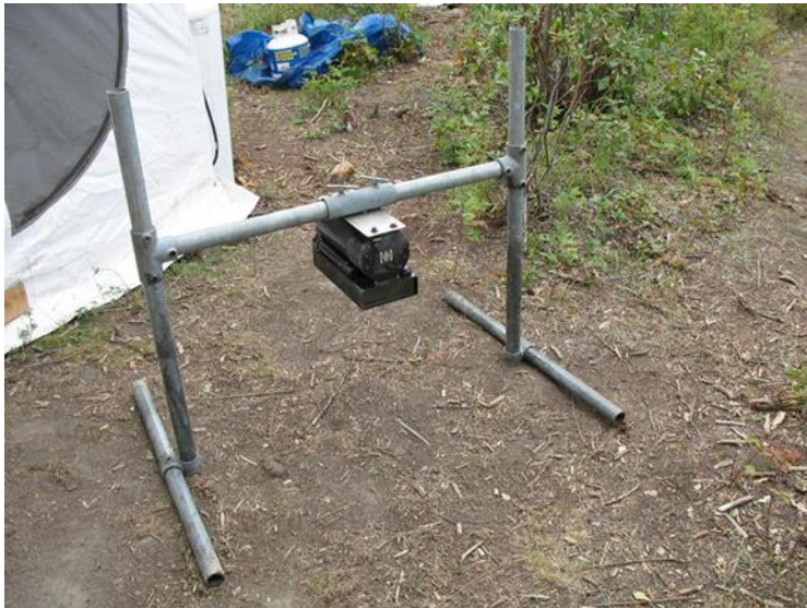
Figure 4. Sonar transducer unit and mounting stand.
