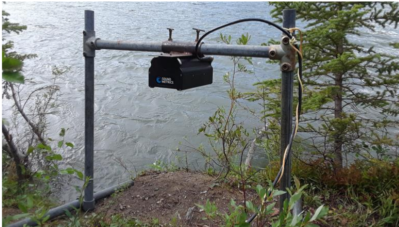
Figure 4. Sonar transducer unit and mounting stand.
