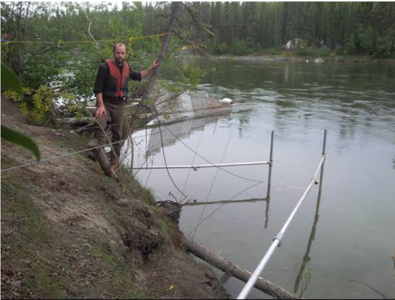
Figure 6. SB sonar unit mounted on stand with diversion fence downstream..
