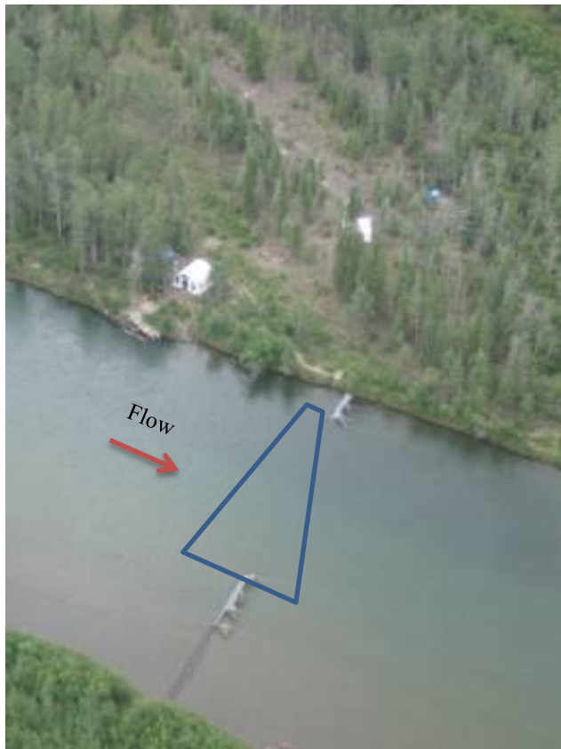
Figure 2. Aerial view of sonar station camp and partial weirs, (photo from 2006 project). Blue outline denotes ensnified portion of the river.
