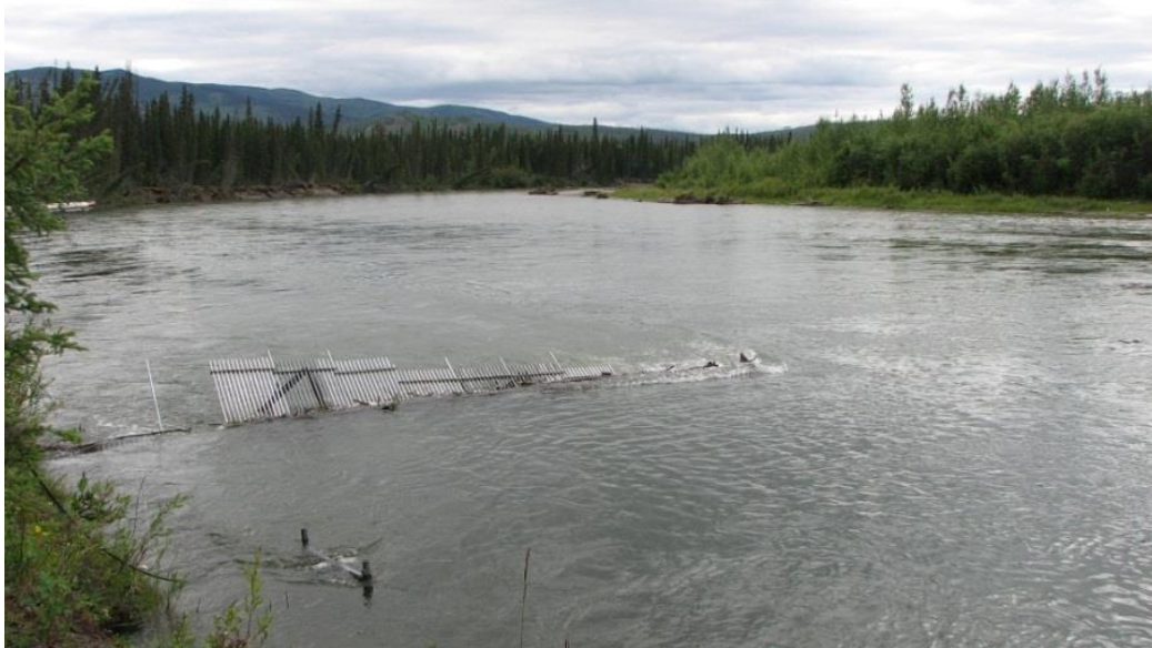
Figure 4. Sonar transducer unit and mounting stand in position. (Photo 2011)
