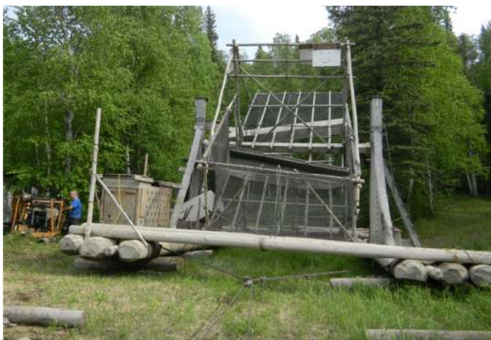
Video wheel ready to be pulled in water by winch at Rapids.
