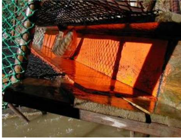
Strategic placement of closed cell foam padding reduces injury dramatically to the fish.
