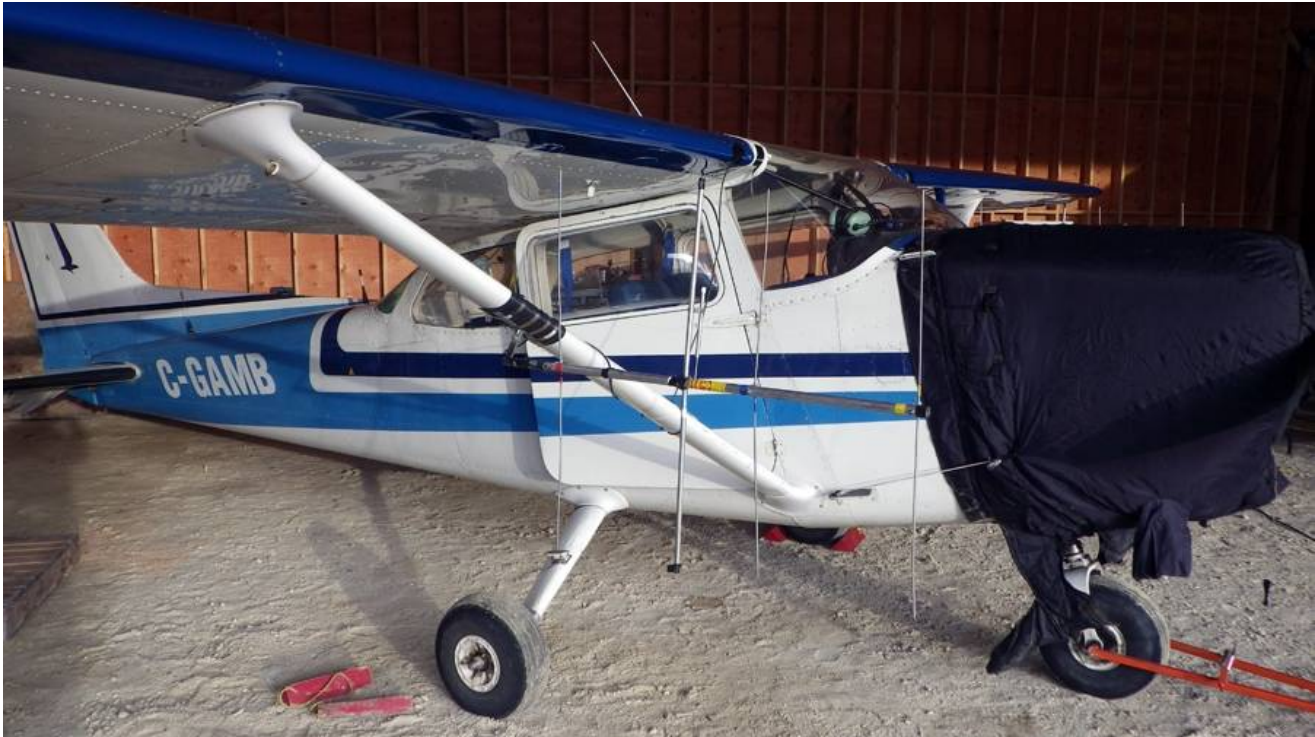
Photo 2. Cessna 172 used during radio telemetry flights, with radio antennas mounted on wing struts. October 12, 2013.
