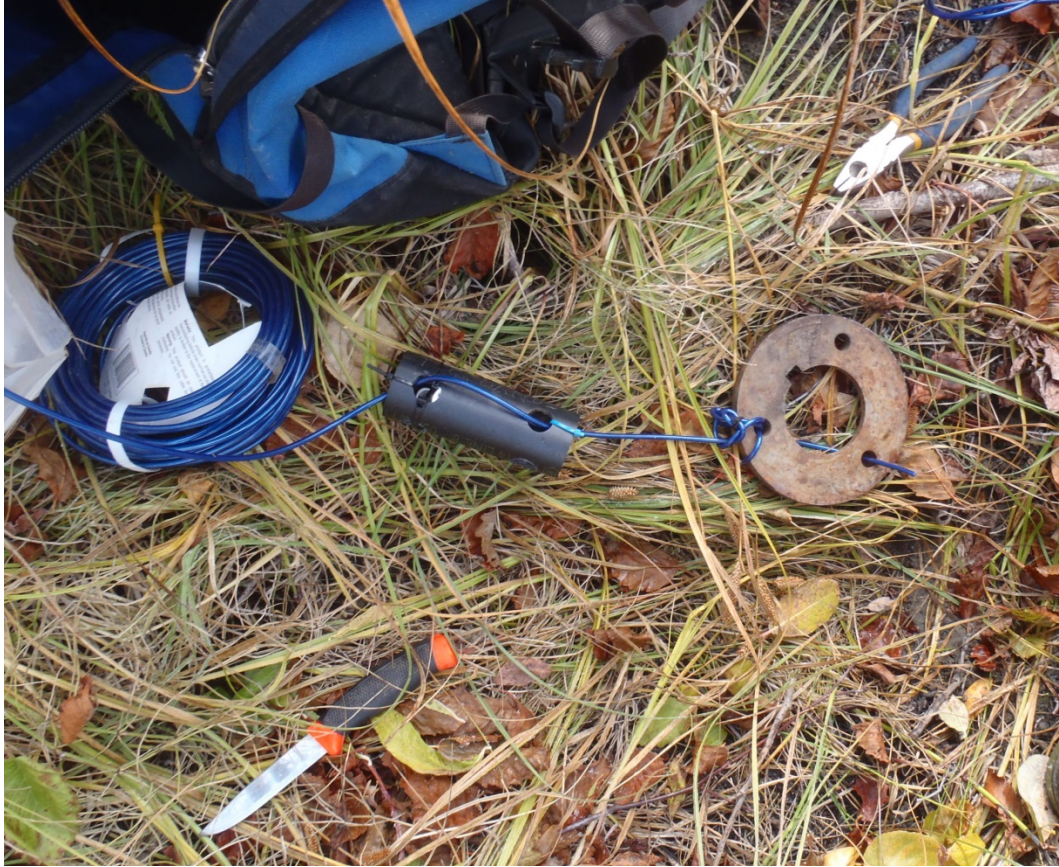
Image 2. Data logger string. The housing is in the center of the image. One logger has been cable tied into the left end of the housing. The second will be cable tied into the right end of the housing. Scrap metal is used as a weight to hold the logger in place.
