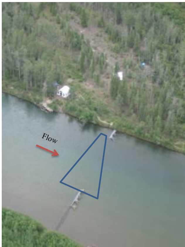
Figure 2. Aerial view of sonar station camp and partial weirs, (photo from 2006 project). Blue outline denotes ensouffled portion of the river.
