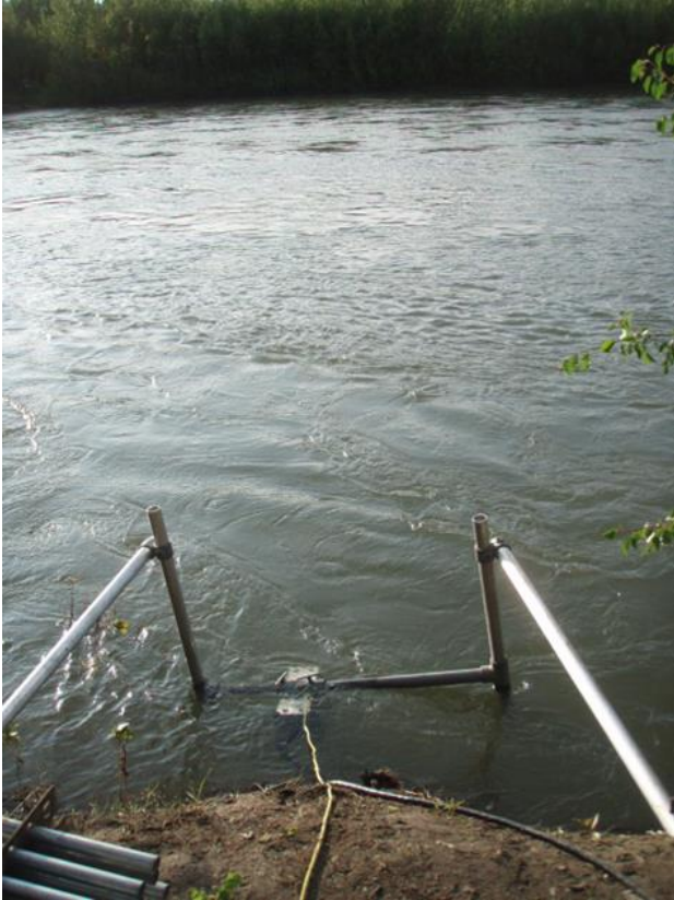
Figure 4. Fabricated sonar stand used in high water.
