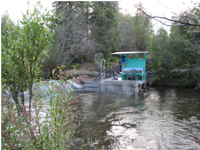
Figure 3. View of counting chamber and sampling station looking from the east bank.
