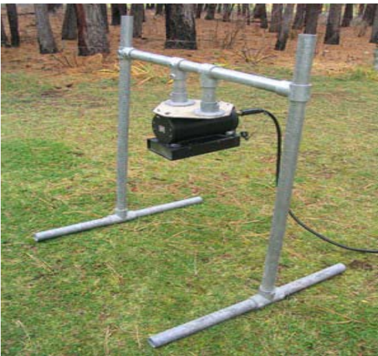
Figure 4. DIDSON sonar unit mounted on adjustable stand.
