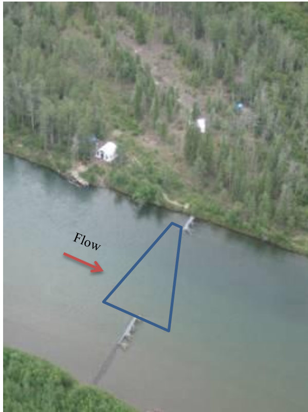
Figure 2. Aerial view of sonar station camp and partial weirs, (photo from 2006 project). Blue outline denotes ensounded portion of the river.
