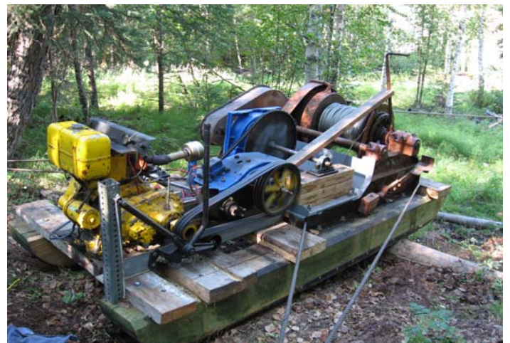
Winch used by project to move wheel in and out of water at Rapids in 2011
