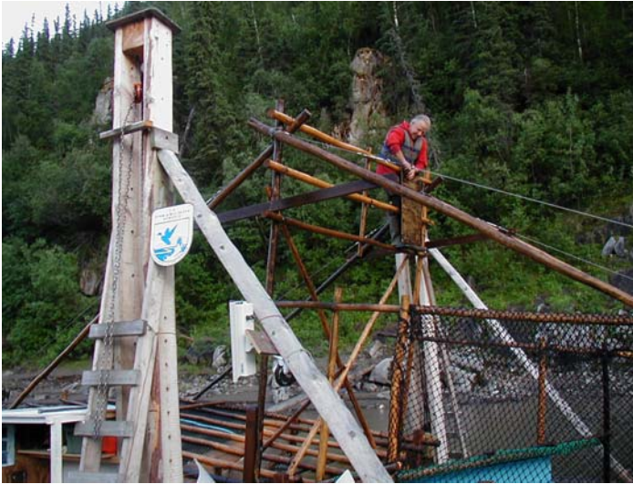
Changing paddle boards to keep wheel rotation slow for fish friendly operation.
