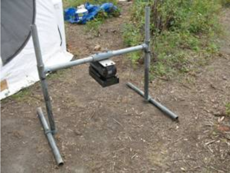
Figure 4. Sonar transducer unit and mounting stand.
