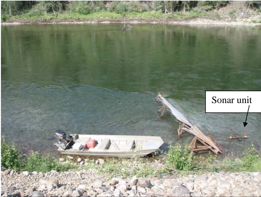
Figure 5. Partial weir structures in place at the Klondike River sonar station, 2010.
