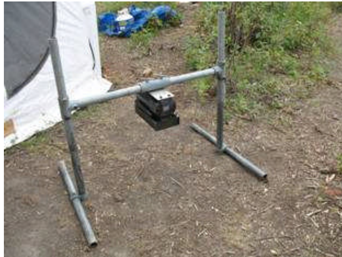
Figure 5. Sonar transducer unit and mounting stand.
