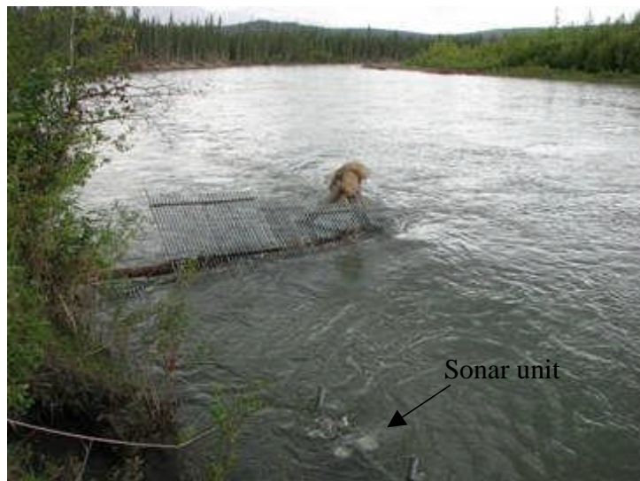
Figure 6. Sonar transducer unit and mounting stand in position.
