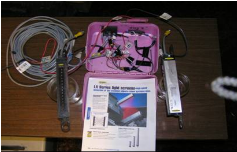
Infrared transmit and receive arrays and control lunchbox
