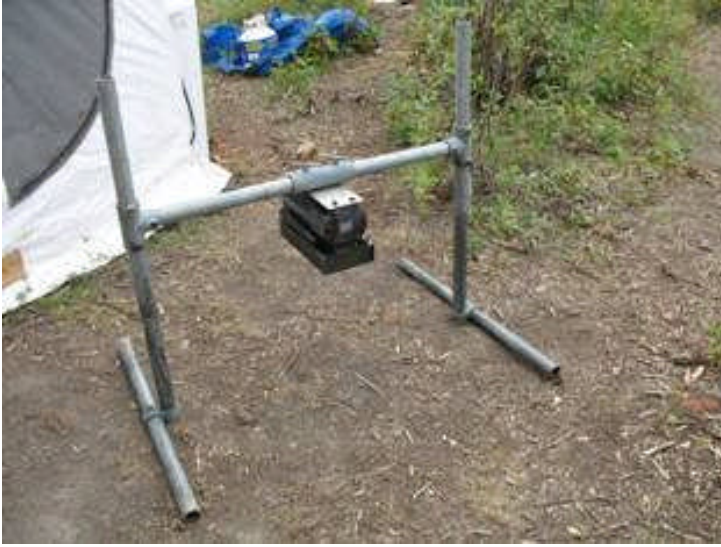
Figure 5. Sonar transducer unit and mounting stand.
